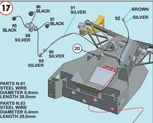
USE PROFILE "A" ON PHOTOCUTTED #1229 TO BEND PARTS 91
