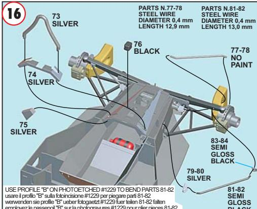
USE PROFILE "B" ON PHOTOCUTTED #1229 TO BEND PARTS 81-82
